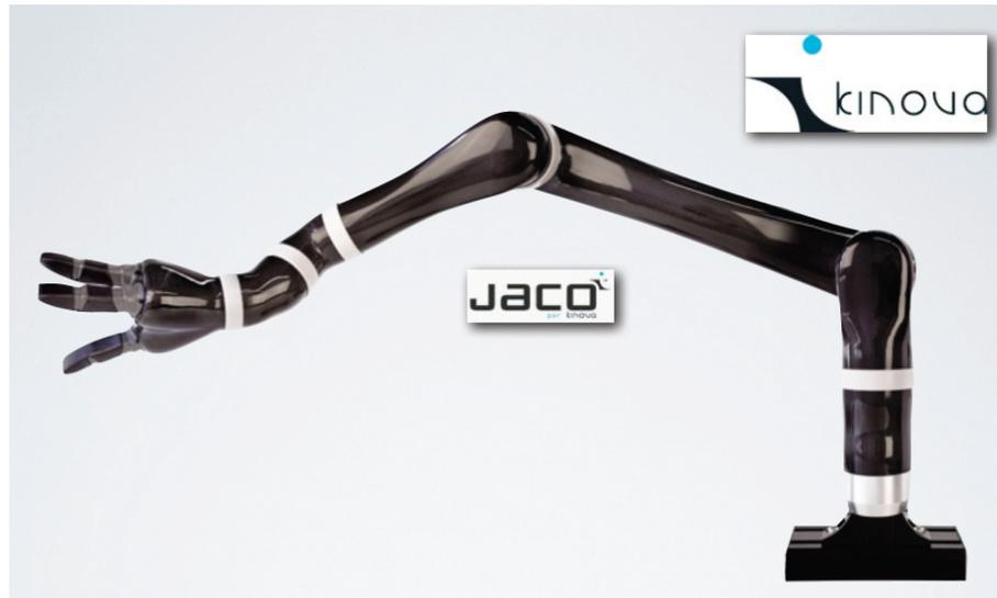
Figure 5: Jaco robotic arm by Kinova.
